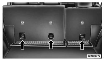
Top Tether Strap Anchorage (Located on Seatback)
